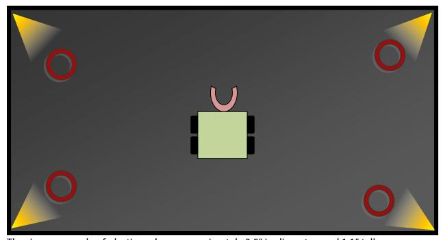
The rings are made of plastic and are approximately 3.5" in diameter, and 1.1" tall.
